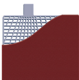
Positive plate example lead dioxide ( \text{PbO}_2 )
